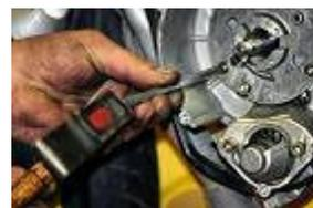
**ATTENTION ! LES 3 VIS DE LA PLATINE SONT PARTICULIEREMENT DIFFICILES A DESSERRE ! POUR SE FAIRE PRESENTER UNE CLE ALLEN DE 3 ET TAPOTER AVEC UN MARTEAU SUR LA CLE**
