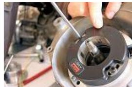
**RECUPERER LE PASSE FIL DU STATOR D'ORIGINE ET LE POSITIONNER DANS BON SENS SUR LA GAINES DU STATOR PREMIUM. PRESENTER LE STATOR PREMIUM SUR LA PLATINE EN PASSANT LA GAINES PAR LE TROU DU CARTER ET LE SERRE AVEC LES 2 VIS 5 X 30 MM FOURNIE.**
